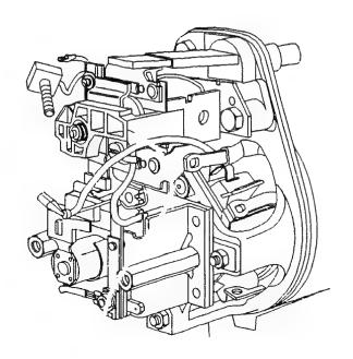
Assembling control relay and starting-motor solenoid
